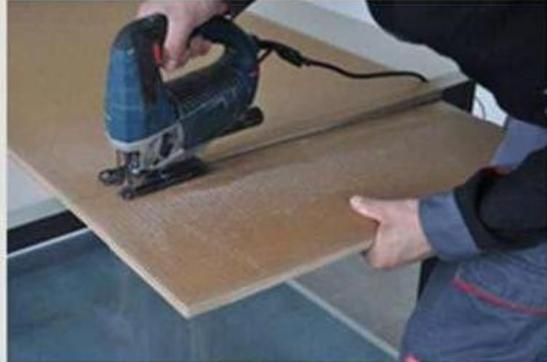
Cut using a jigsaw with a metal or ceramic blade, or a fine toothed circular saw blade.
